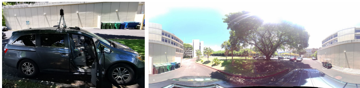
Fig. 1. (Left) A MCS system with a 360-degree camera mounted on top of a vehicle. (Right) An example panoramic photo captured by the MCS.
